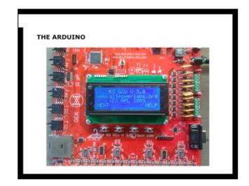
Here's one from All Power Labs that's used for precisely controlling an alternative energy gasifier unit.
