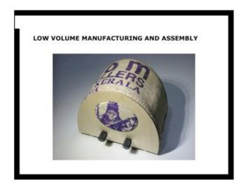
This is a digital radio that David Mellis did as part of his MIT Media Lab master's thesis last year. It's designed to be a base design that can be quickly iterated on and to use cheap materials. Dave is one of the developers of the Arduino, and he intentionally made a very technologically simple product to focus on the core ideas of lightweight manufacturing and rapid iteration.
